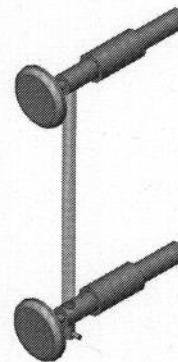
Figure 6.4: Gauge Glass Installation
